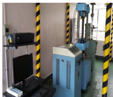
Fig. 2 Universal Testing Machine
