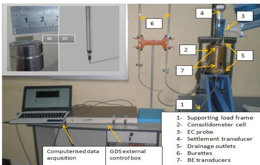
Figure 1: Instrumented Consolidometer Set Up
