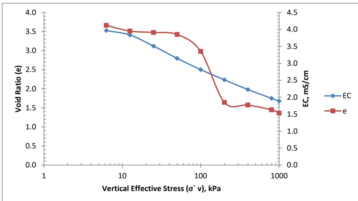
Figure 5: Void Ratio (e) vs EC With Respect to Vertical Applied Stress ( $\sigma_v$ )
