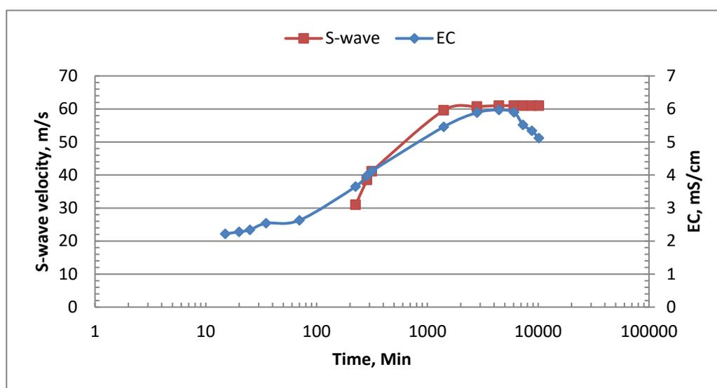
Figure 2: S-wave and EC behaviour during the Curing time
