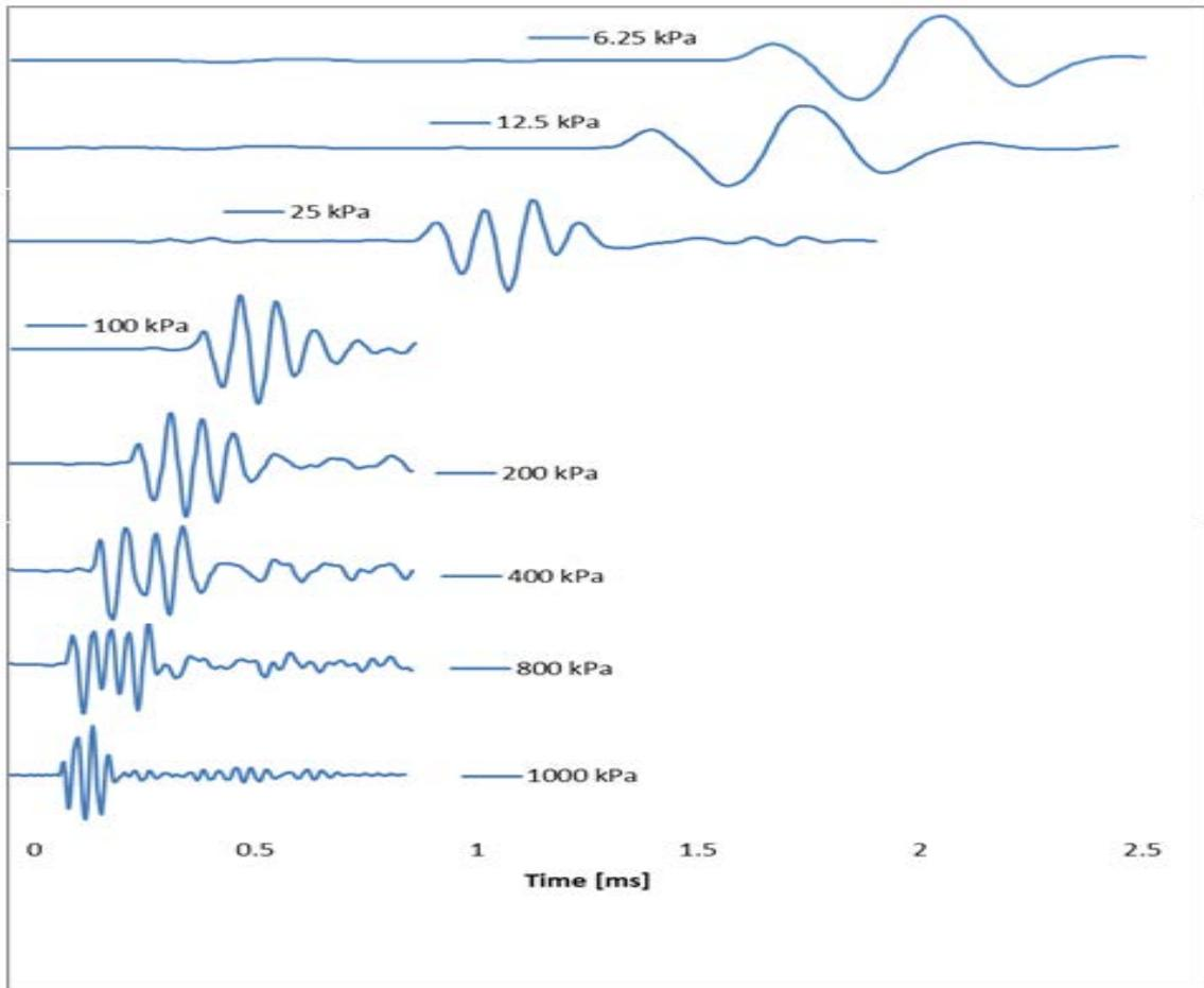
Figure 4: Typical S-Wave Response for Different Stresses
