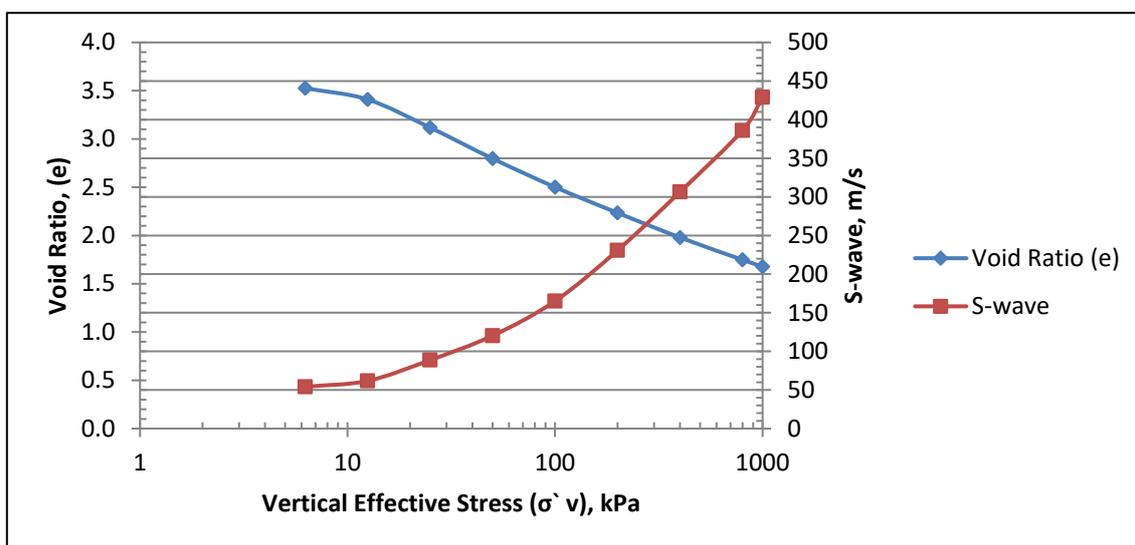
Figure 3: Void ratio (e) vs S-wave With Respect to Vertical Applied Stress ( $\sigma'_v$ )
